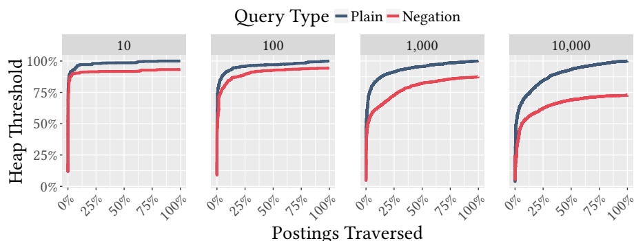
Fig. 3: Comparing the heap threshold of the negated query to the heap threshold of the plain query for the query pair “silver city -new mexico” and “silver city mexico”. Clearly, by negating documents containing the term new , fewer high scoring documents make it into the heap, leading to a reduced threshold, and less ability for dynamic pruning to occur. As k increases, so too does the gap between the plain and negated threshold.
