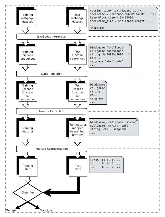
*Figure 5.7:* Opcode *data processing, reduction, transformation, and classification.*
